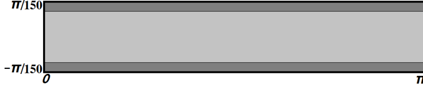
FIGURE 1. The plate \Omega and its subset (dark grey) where the cables+hangers act.
