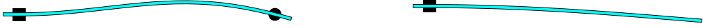
Figure 1: The depicted boundary condition for the left endpoints of these two cross sections is clamped , while the boundary conditions for the right endpoints are respectively hinged and free .
